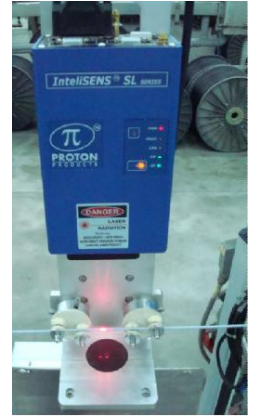
Tube: 1 x SL1525 with PHA2 mounting console
