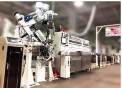
**In 2014** - "45+25+35 skin-foam-skin nitrogen injection physical foaming insulation extruder line" developed in GEMWELL, solved bottleneck of insulation process production of data cable in small specifications, selling both in China and abroad.
